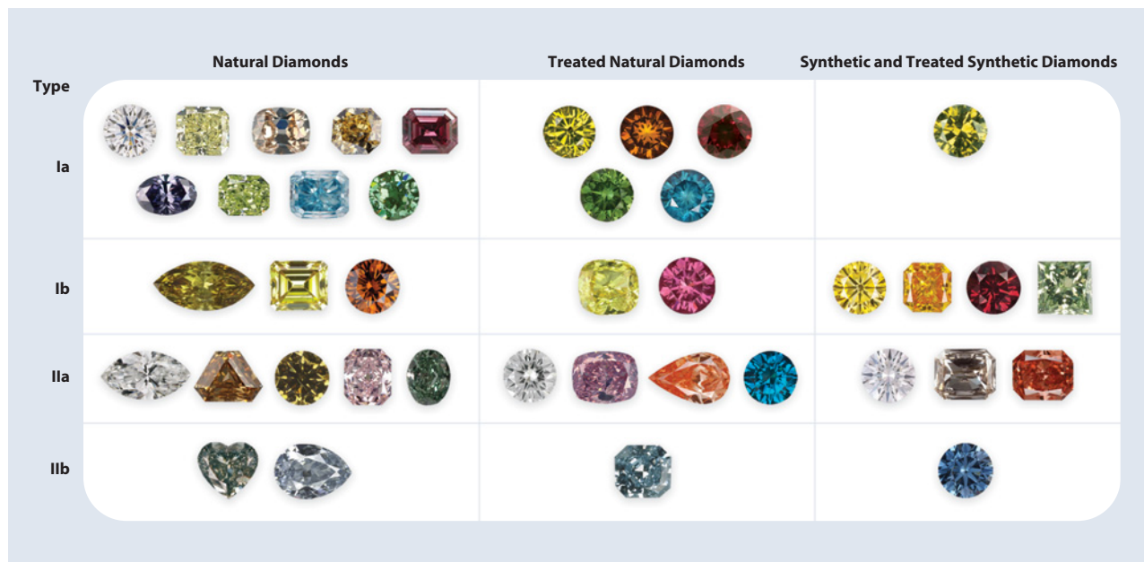
Figure 3. Color is strongly influenced by the impurities/defects in the diamond lattice. Consequently, diamond type plays an important role in the potential colors of natural, synthetic, and treated stones. Although much experience is necessary to even attempt an assessment of diamond type using color observations, these images show some of the representative colors for each category. Photos by various GIA staff.
