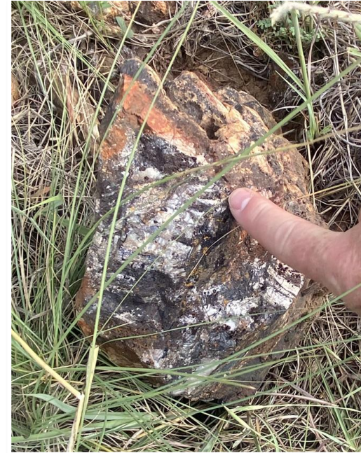
Target A: altered BIF, vicinity of KR25-157; example of discordant quartz flooding, veining, evidence of weathered sulphide
